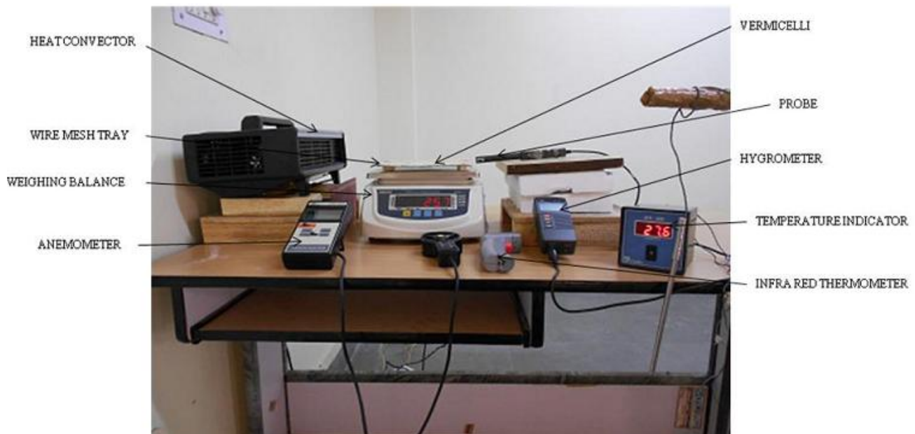
Figure 1: A photograph of experimental set-up for indoor forced convection drying mode
